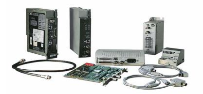
The ControlNet network is a real-time control network that provides high-speed transport of both time-critical I/O and interlocking data and messaging data, including upload/download of programming and configuration data on a single physical media link. The ControlNet network's highly efficient data transfer capability significantly enhances I/O performance and peer-to-peer communication in any system or application where it is used.
